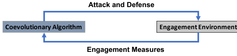
Fig. 7: High level view of RIVALS framework. The left hand side component is a competitive coevolutionary algorithm that evolves two competing populations: attacks and defenses. The right hand side component from a computational perspective is a modeling or simulation environment. The environment is initialized with a mission and can be reset each time it is passed an attack-defense pairing to run an engagement. It first installs the defense, then it starts the mission and the attack. It evaluates the performance of the adversaries relative to their objectives and returns appropriate measurements.
